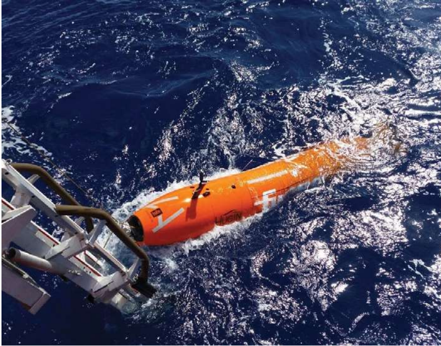
LEFT: Fugro's Echo Surveyor VII is specifically designed for high resolution and efficient survey operations in water depths reaching 4,500 metres.
